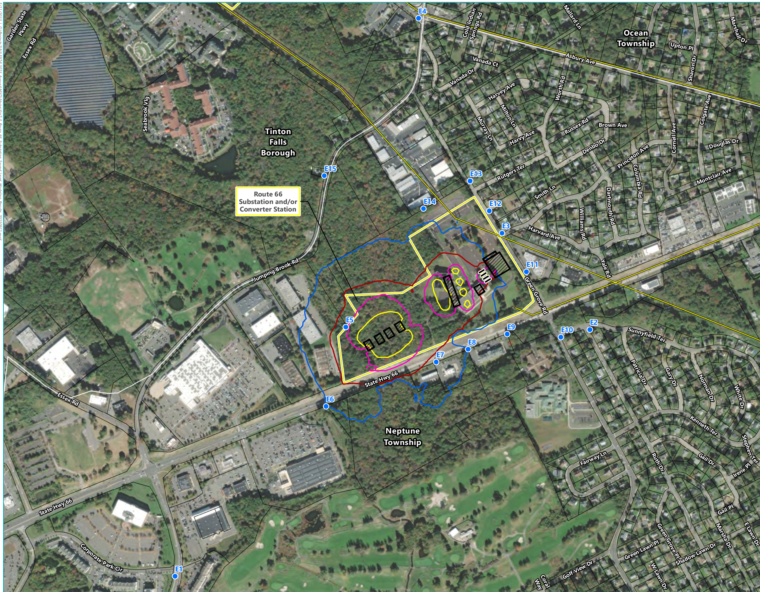
Figure 7-5 Proposed Onshore Substation and/or Converter Station – Route 66 Site Sound Level Modeling Results Monmouth County, New Jersey
