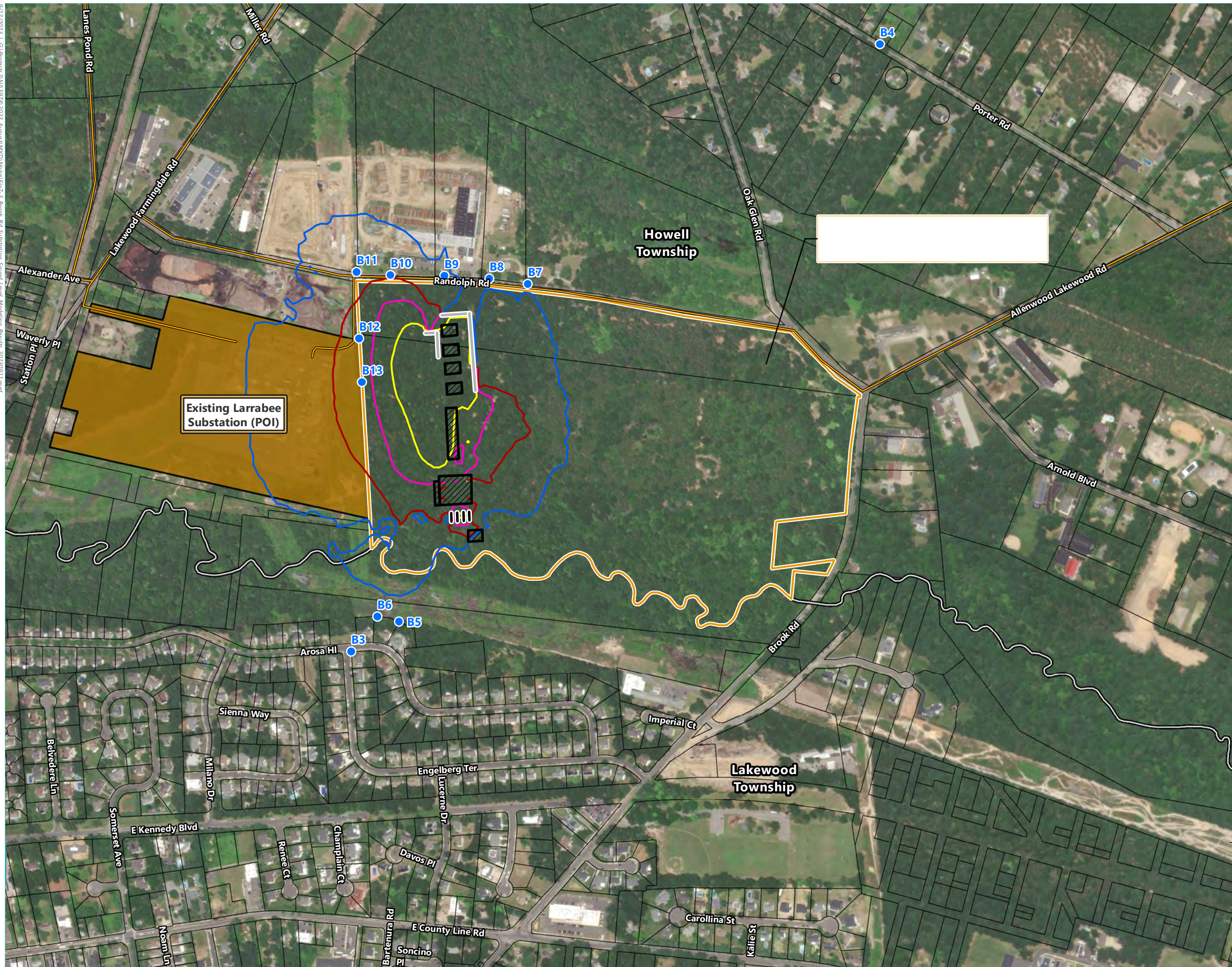
Figure 7-3 Proposed Onshore Substation and/or Converter Station – Brook Road Site Sound Level Modeling Results Monmouth County, New Jersey
