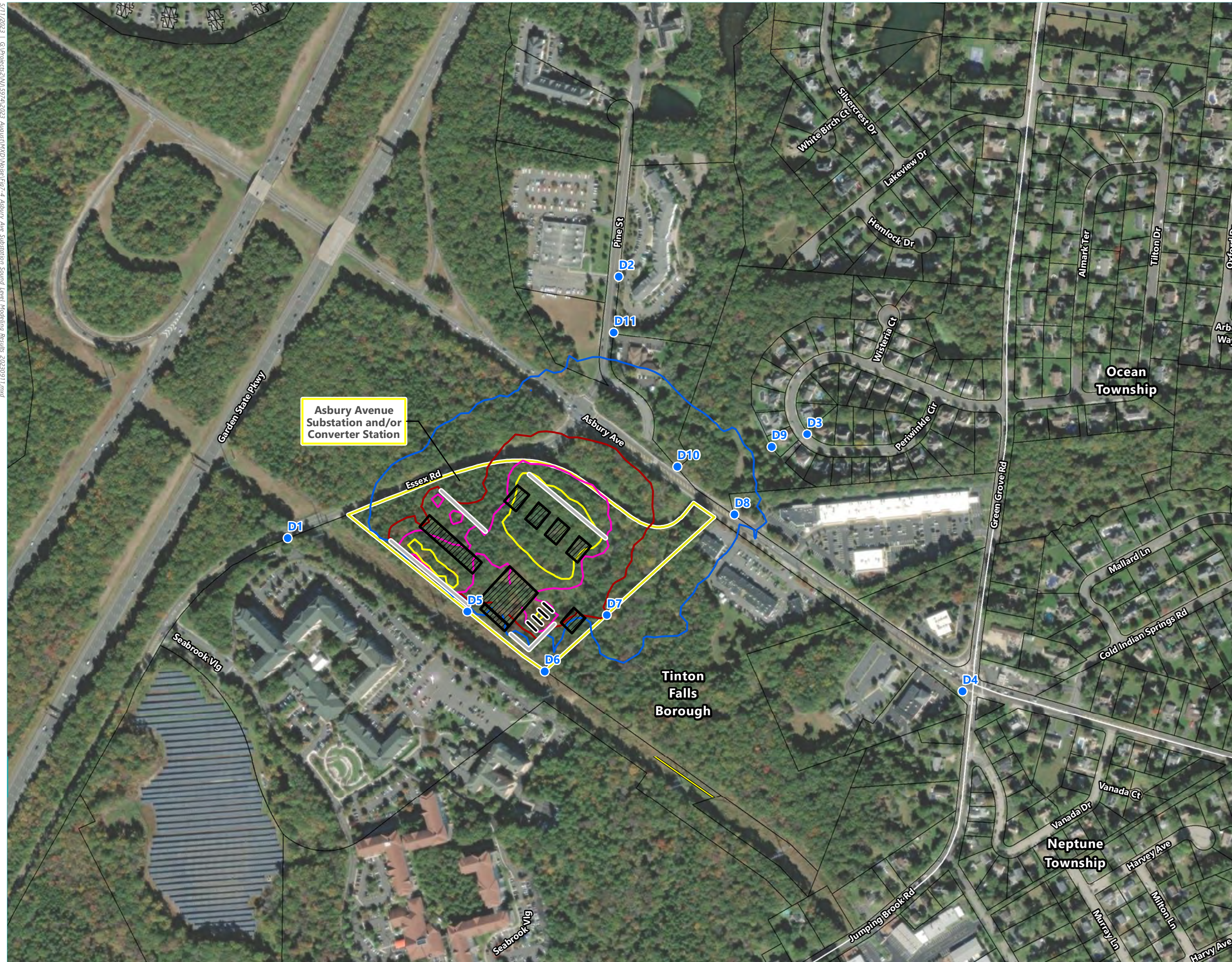
Figure 7-4 Proposed Onshore Substation and/or Converter Station – Asbury Avenue Site Sound Level Modeling Results Monmouth County, New Jersey
