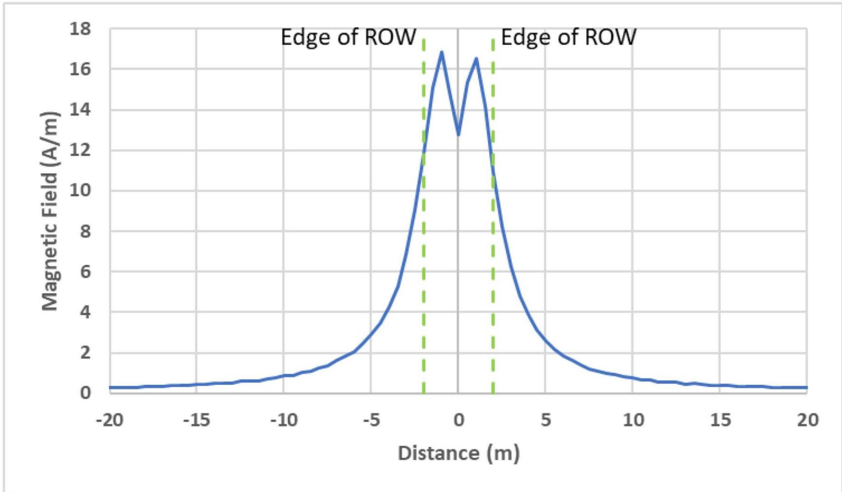
**Electromagnetic Field (EMF) Assessment, Case 42:** Magnetic field results at the surface for 230 kV high voltage alternating current (HVAC) onshore interconnection cables (four circuits, 3,000 mm<sup>2</sup> Cu single core) installed underground in a narrow right-of-way corridor.
