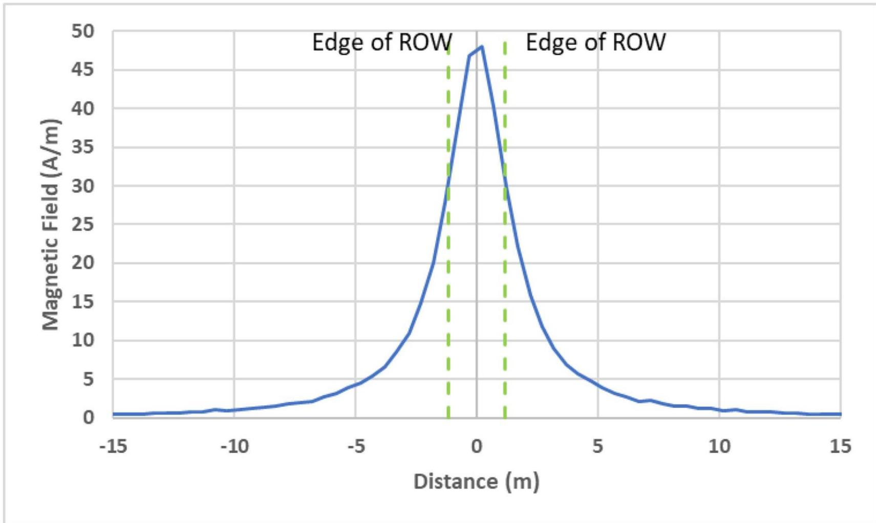
**Electromagnetic Field (EMF) Assessment, Case 48:** Magnetic field results at the surface for 320 kV high voltage direct current (HVDC) onshore interconnection cables (one circuit, 2,500 mm<sup>2</sup> Cu) installed underground.
