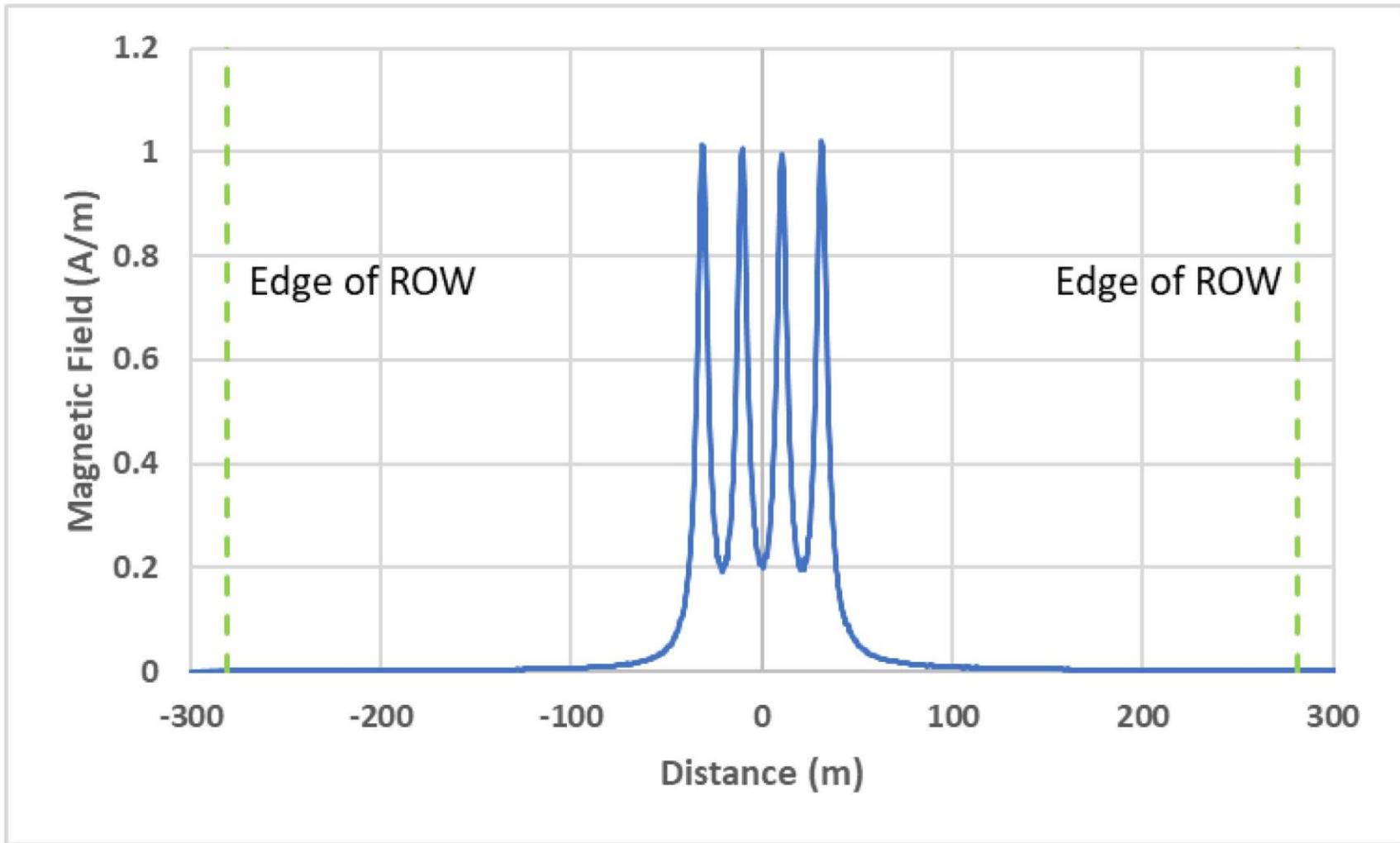
**Electromagnetic Field (EMF) Assessment, Case 29:** Magnetic field results at the seabed for four 230 kV high voltage alternating current (HVAC) export cables (2,000 mm<sup>2</sup> Cu) installed via horizontal directional drilling at the landfall sites.
