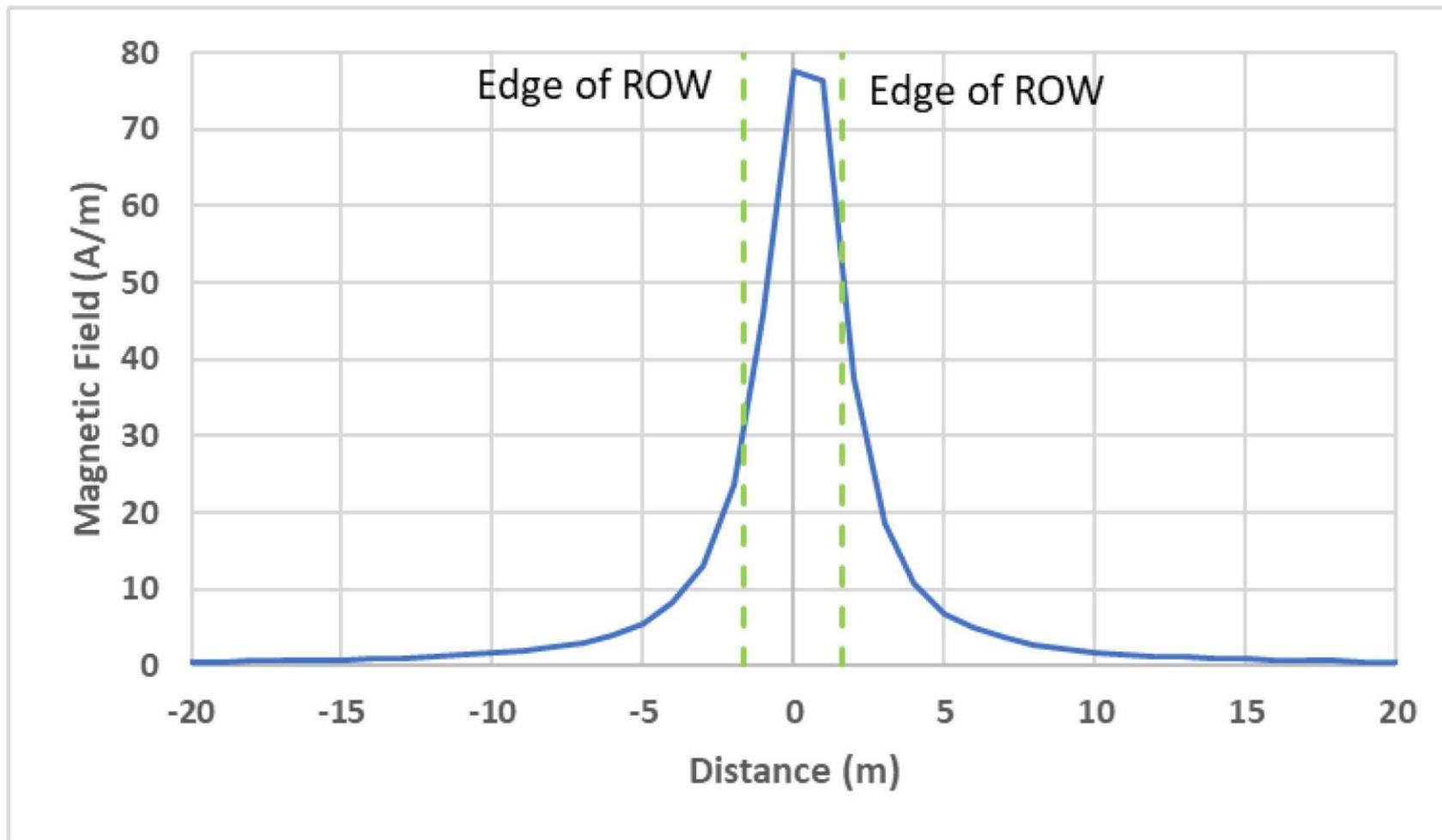
**Electromagnetic Field (EMF) Assessment, Case 46:** Magnetic field results at the surface for 275 kV HVAC Onshore interconnection transmission cables (3000 mm<sup>2</sup> Cu Single Core) and 525 kV HVDC Onshore interconnection transmission cables (2500 mm<sup>2</sup> Cu) installed underground and operating in monopole mode.
