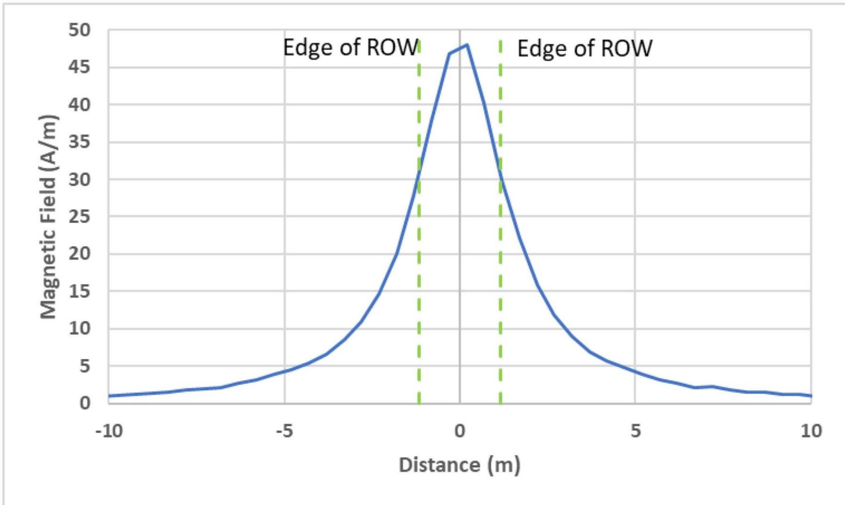
**Electromagnetic Field (EMF) Assessment, Case 52:** Magnetic field results at the surface for 525 kV high voltage direct current (HVDC) onshore interconnection cables (2,500 mm<sup>2</sup> Cu) installed underground and operating in monopole mode.
