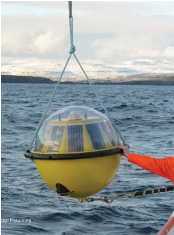
Figure 2 - Axys Technologies Triaxys wave buoy ( http://axystechnologies.com/products/triaxys-directional-wave-buoy/?open_cat=40 ).
