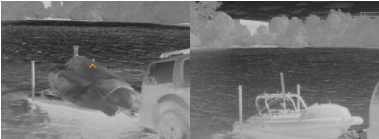
Figure 2. Thermal image of the USV Babou with (left) and without (right) the tarp. Both images collected during daylight.
