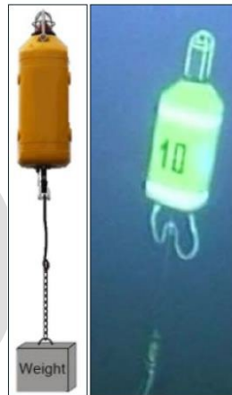
Figure F-2: Example of Underwater Positioning Transponder with Floatation Collar attached to a Weight
