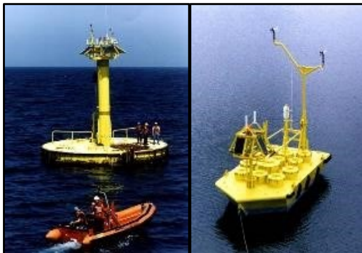
Figure 2-2: Ten Meter Discus-Shaped Hull Buoy (left); Six Meter Boat-Shaped Hull Buoy (right)
