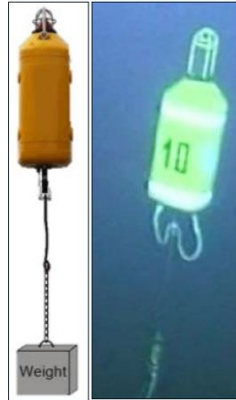
Figure A-2: Example of Underwater Positioning Transponder with Floatation Collar attached to a Weight
