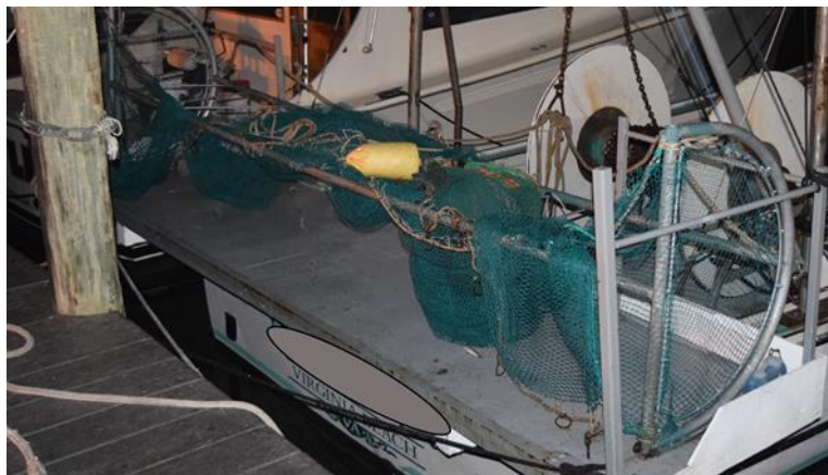
Figure W-34. Beam Trawl, 16 Feet in Width, Secured to the Stern of a Fishing Vessel in Rudee Inlet (Photo Credit: R. Larsen Sea Risk Solutions, LLC)
