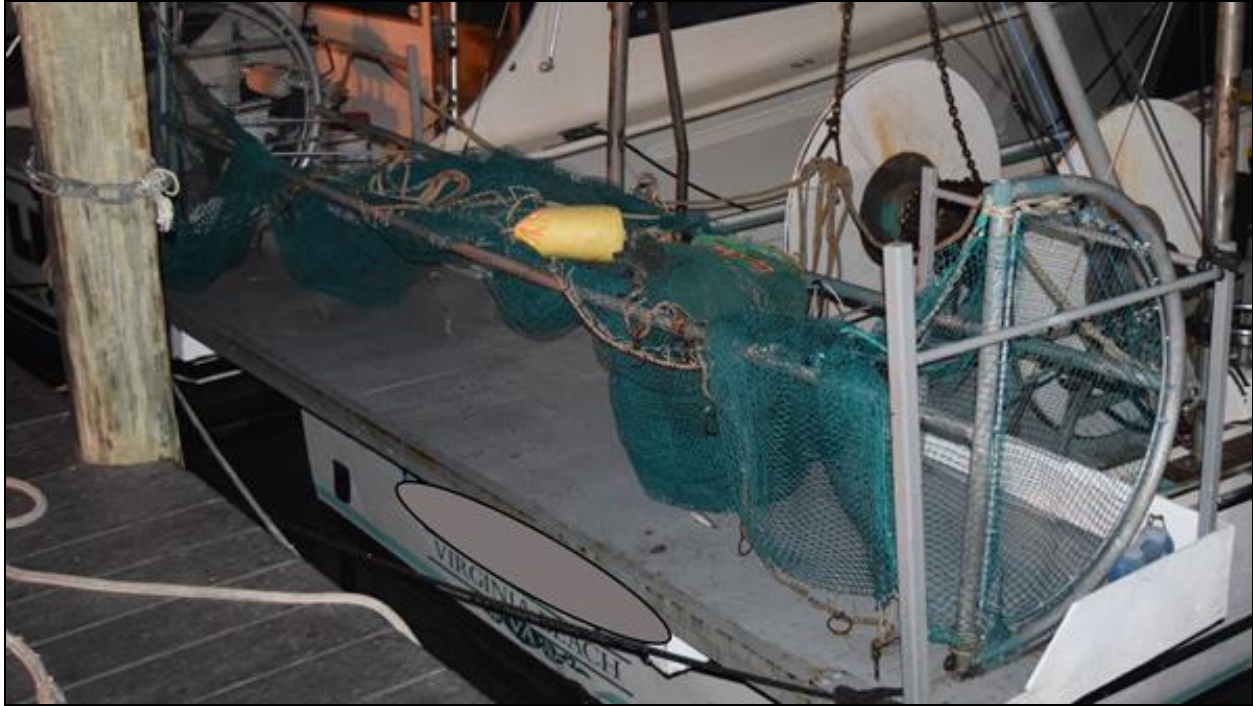
Figure 4.4-42. Beam Trawl, 16 feet in width, Secured to the Stern of a Fishing Vessel in Rudee Inlet
