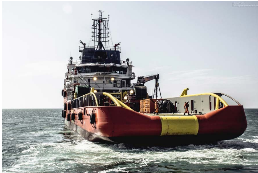
Figure 14. Anchor-handling tug supply vessel used for mooring and anchor installation activities.
