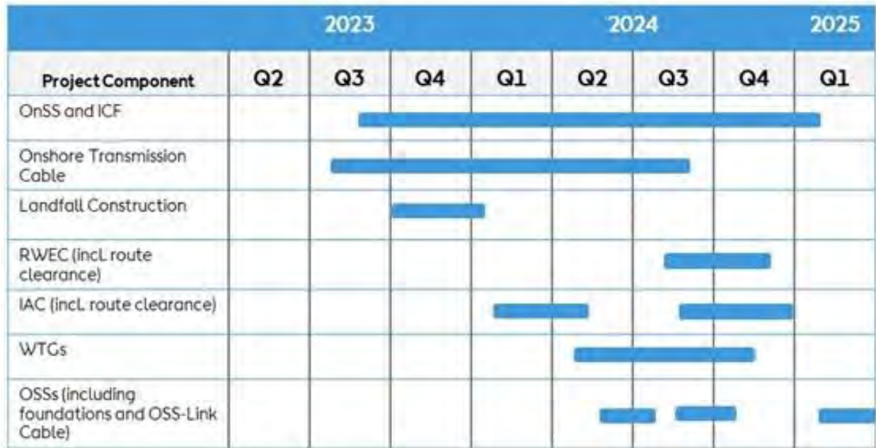
Figure 2.1-9. Revolution Wind Farm indicative construction schedule (VHB 2023).
