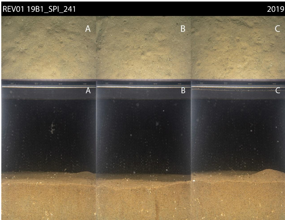
Figure 2-11. Schematic diagram of the operation of the sediment profile and plan view (SPI/PV) camera imaging system; the PV camera images an area of ~1 m 2 and the SPI camera images a profile of the sediment column that is 14.5 cm across and up to ~21 cm high. Three replicate images are analyzed at each station and a composite of these three paired replicate PV images (top) and SPI images (bottom) is prepared for use in reporting products.
