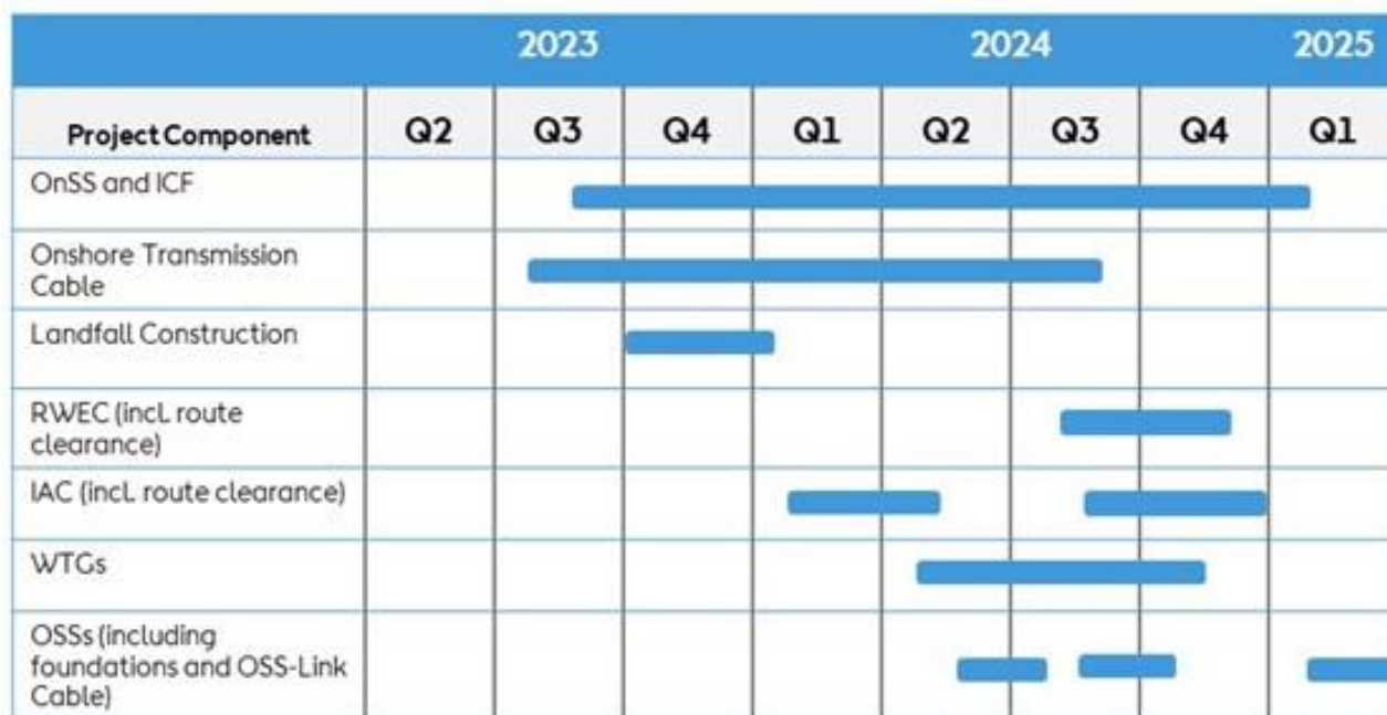
Figure 1. Indicative construction schedule for the Revolution Wind Farm and Revolution Wind Export Cable.
