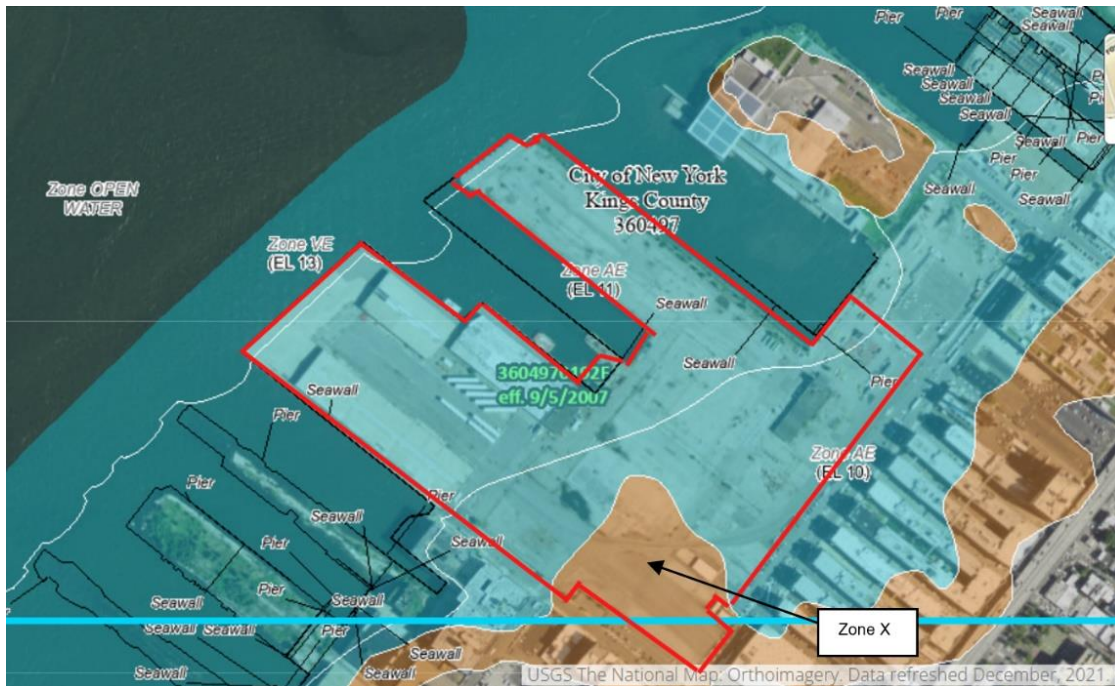
Figure 3.9-1 FEMA Flood Zones Within and Adjacent to the Terrestrial Project Area. Zone AE = 1 Percent Annual Chance of Flooding, Zone X = 0.2 Percent Chance of Flooding.
