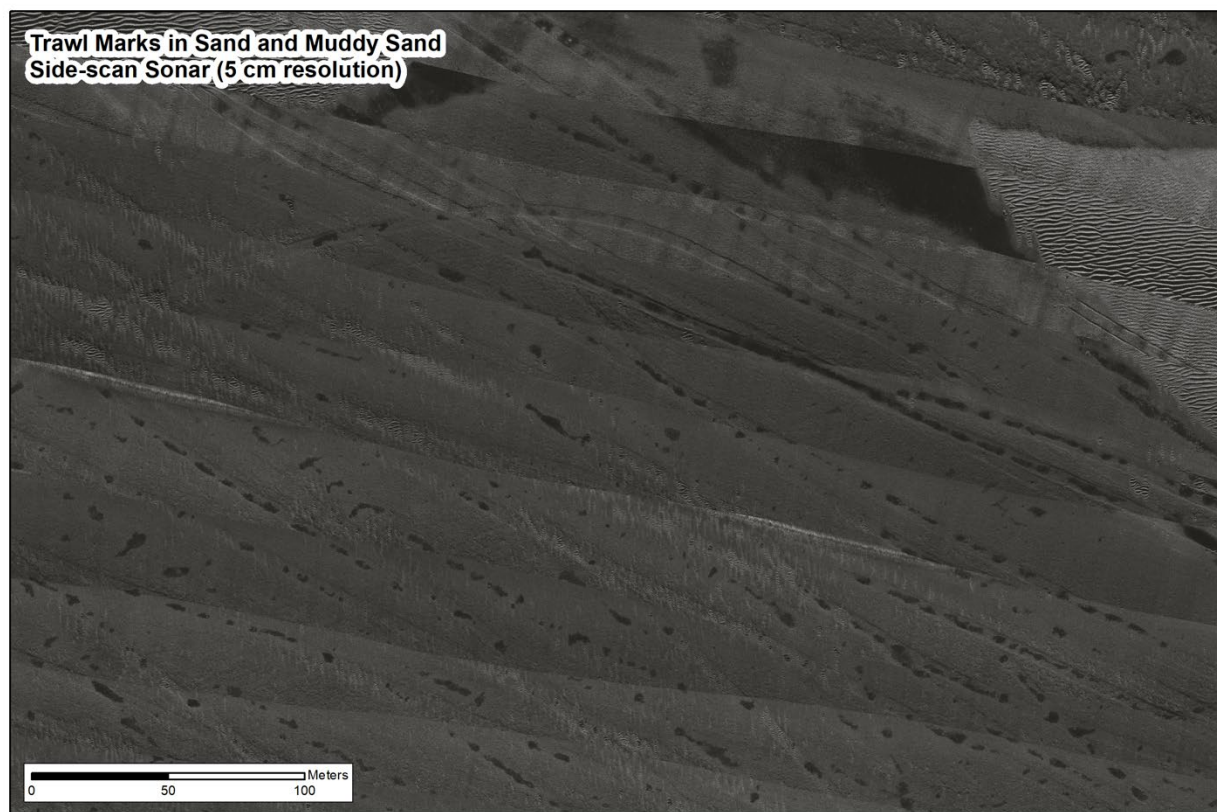
Figure 17. Side-scan sonar data in an area of Sand and Muddy Sand at the SRW Project area, demonstrating high fishing activity as evidenced by numerous trawl marks across the sediment surface.
