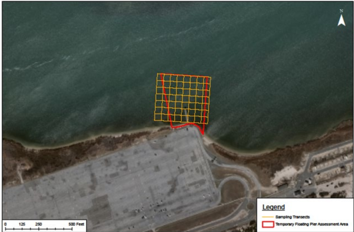
Figure 3-19. Sampling grid used for Sunrise Wind SAV survey of the proposed temporary landing structure and vicinity. Transects run east-west and north-south and are spaced approximately 50 feet apart.
