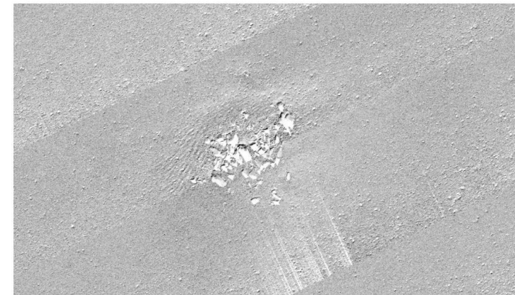
Side scan sonar image of a potential shipwreck site on the Outer Continental Shelf.
