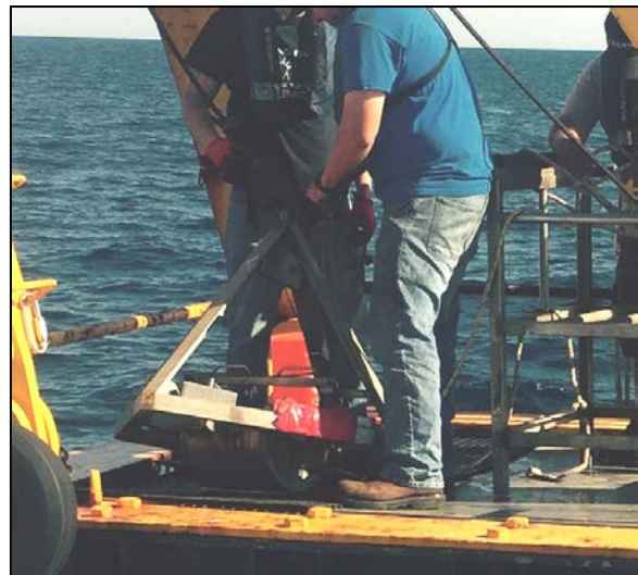
Preparing Van Veen grab sampler on R/V Shearwater
