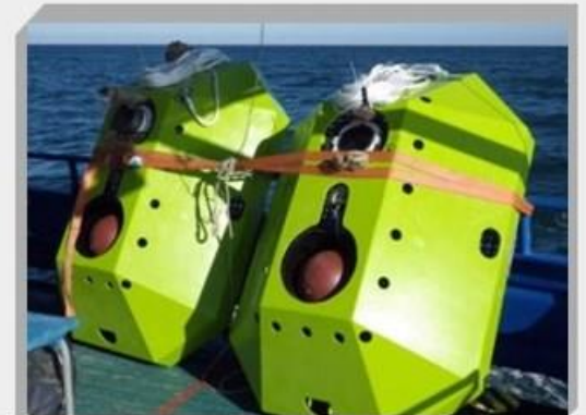
Above: General Purpose GP-TRBM system manufactured by MSI
