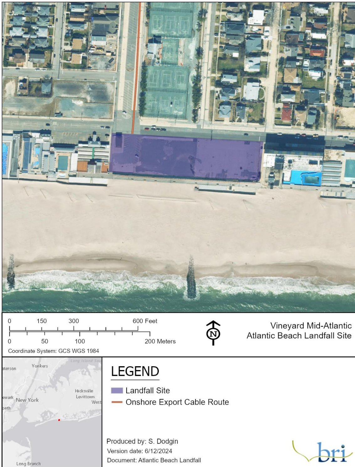
Figure 3-4: A potential landfall site in a paved parking area near Atlantic Beach in the Town of Hempstead, New York.
