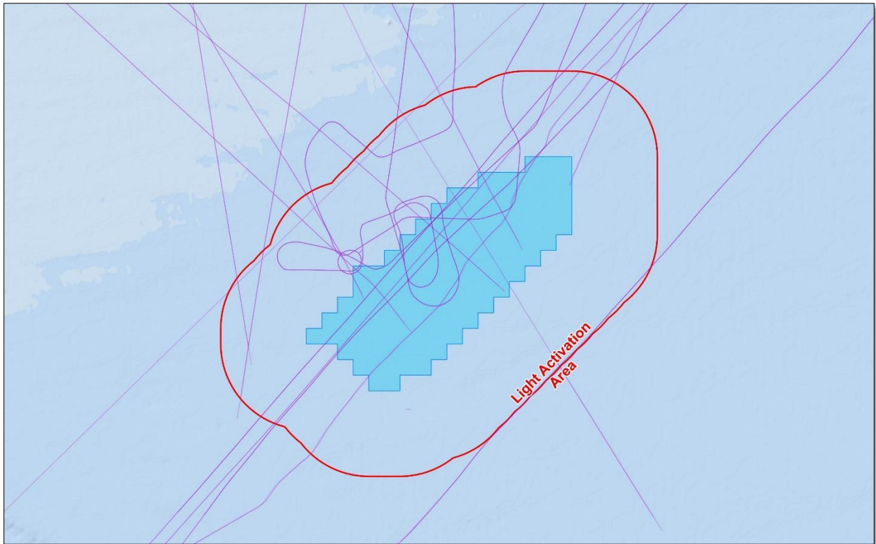
Figure 3: Flight tracks (purple) with more than one radar return that would have activated ADLS obstruction lights (based on 1,165-foot (355-meter) tall wind turbines)
