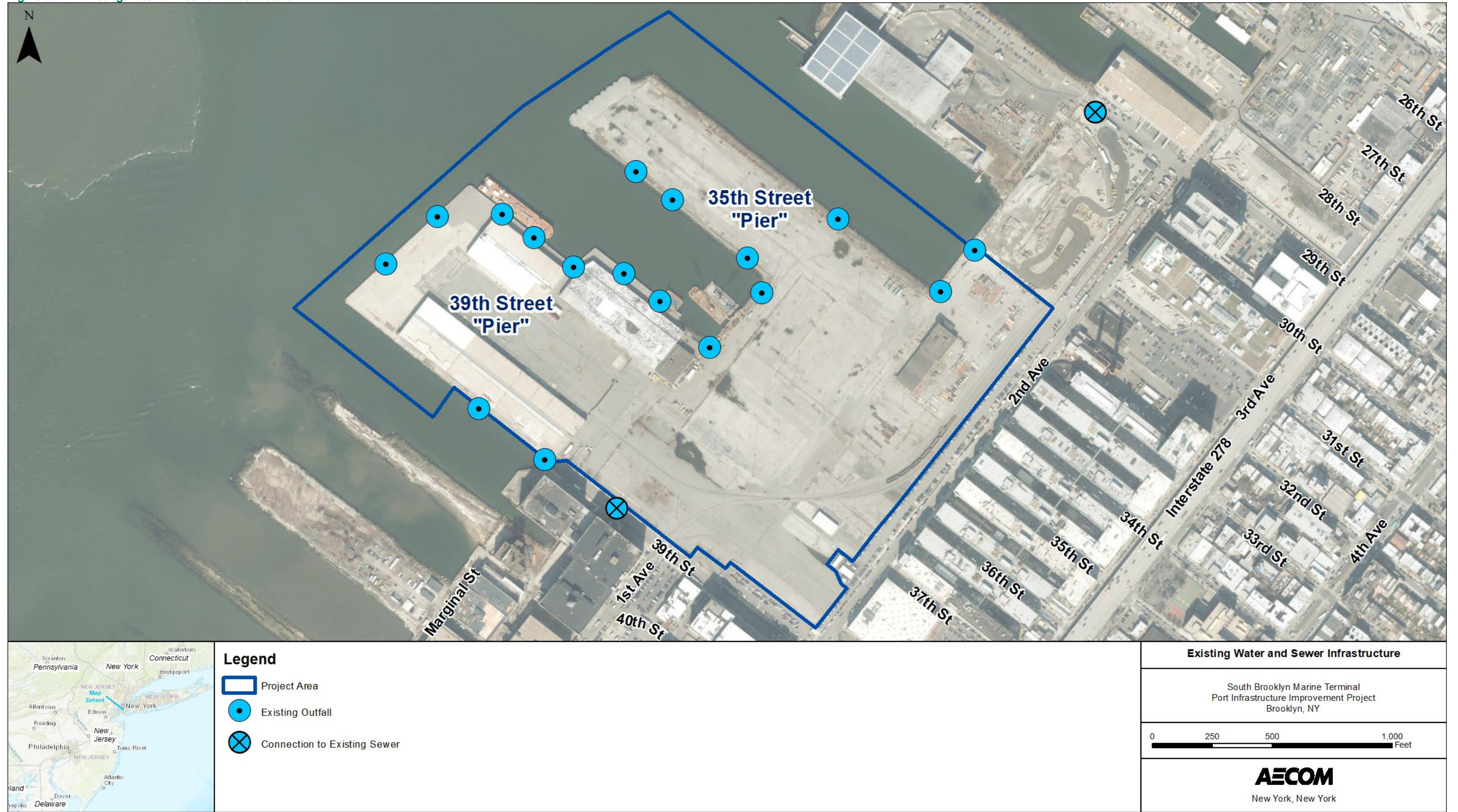
Figure 3.11-1 Existing Water and Sewer Infrastructure
