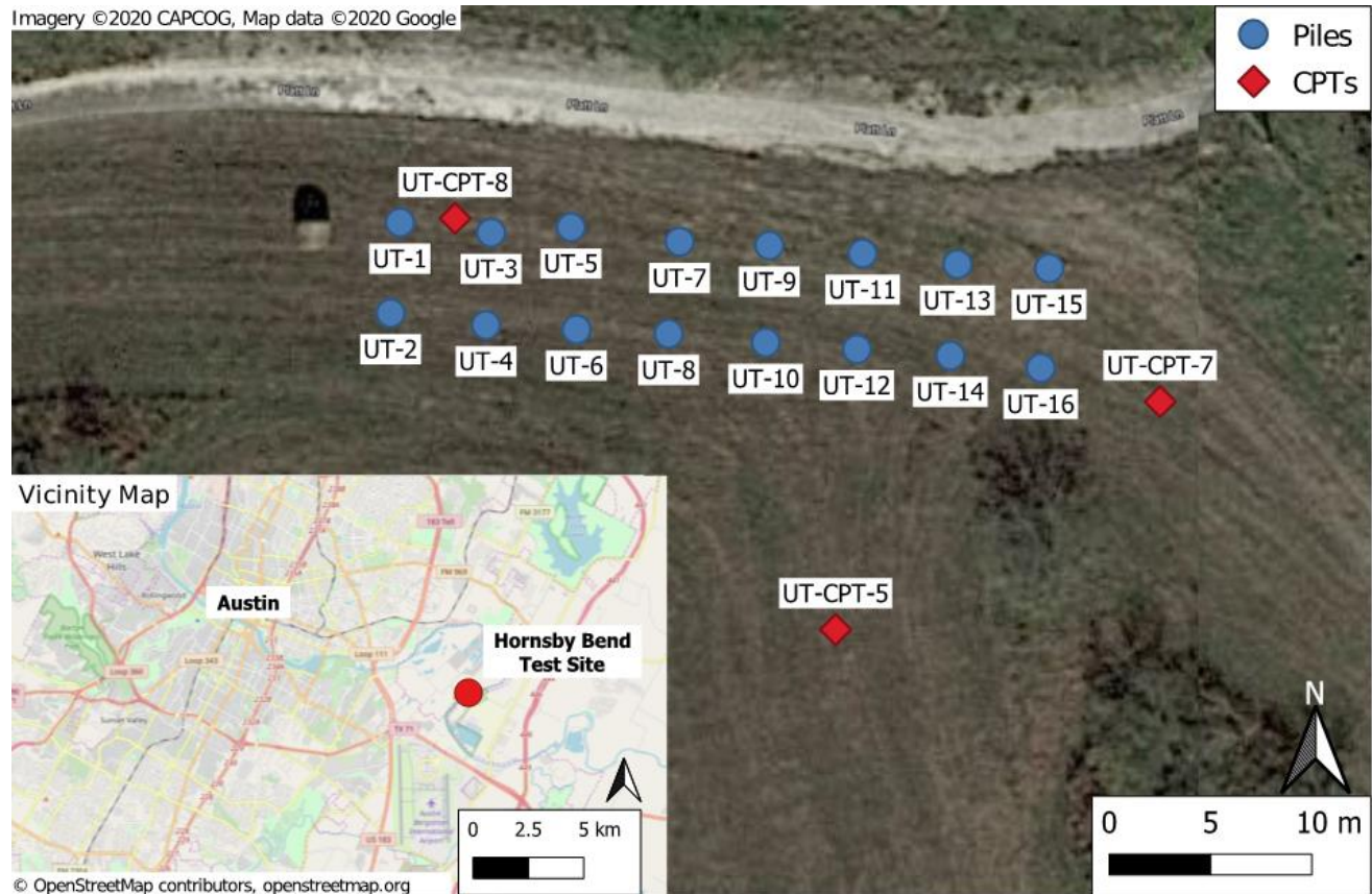
Figure 2-9 Site plan of geotechnical investigations and pile testing at the UT test site
