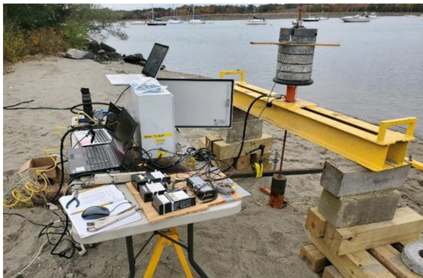
Figure 4-1 Photograph of a typical pile load test setup at the URI test site
