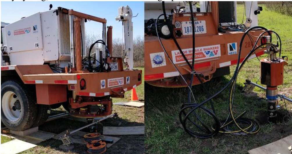
(a) shaker truck load applied to pile
