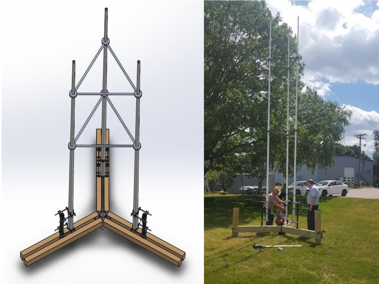
Figure 2.7. System using three Shakespeare 476 Classic VHF antennas 6.4 m omnidirectional antennas used for phase delay estimation of bearing from receiver to a tagged organism. Dr Jim Miller (r), Fred Pease (l), and Jesse Moore (c – kneeling) are shown during construction.
