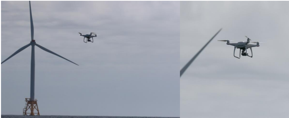
Figure 1.19. Quadcopter drone during calibration surveys within 1 km of the Block Island Wind Farm. Right panel: Nanotag was taped to right lower strut of quadcopter.
