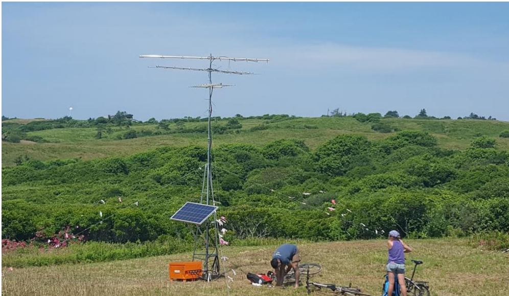
Figure 1.9. Telescoping mast (~6 m tall) used at Black Rock and Southeast Lighthouse, Block Island, RI during 2017 field season. This photo is the Black Rock station with three 9-element 3.3 m long, 11-dB Yagi antennas, a 140-watt solar panel used as power source, and metal lockable tool case that contained the receiver, solar charge controller and 2 marine batteries.
