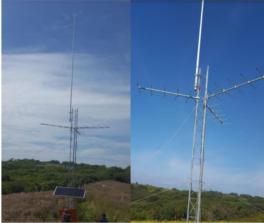
Figure 1.10. Tower array at Black Rock, Block Island used during 2018 field season, which consisted of two 3.3 m tower segments with three 5-element 8-dB Yagi antennas and one 6.4 m tall 10-dB omnidirectional antenna.
