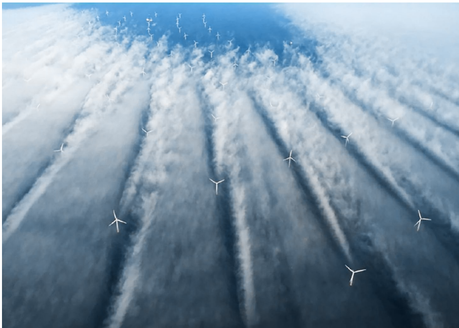
Photo: Horns Rev 2 Visible Wakes (Hasager, et al., 2017). Wind Farm Wake
