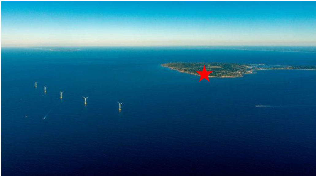
Figure 1.17. Block Island Wind Farm, five 6-MW turbines ~5 km off Block Island, started operations were initiated on 12 December 2016. Since 2015, an automated radio telemetry station at SE Lighthouse (red star) has tracked birds with digital VHF transmitters. Turbine #1 (far right turbine) had a VHF telemetry receiving station in 2017 to 2019. Photo courtesy of dwwind.com
