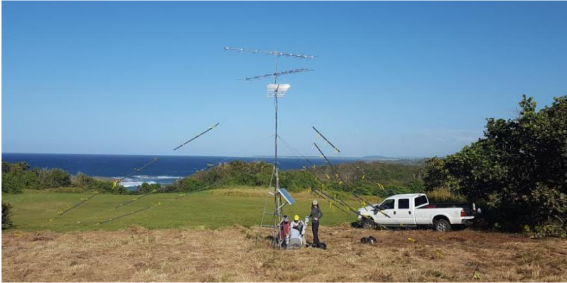
Figure 1.7. Example of a Motus Wildlife Tracking System station with three 9-element, 11-dB Yagi antennas located on a 6 m telescoping mast on the northcentral Puerto Rico.
