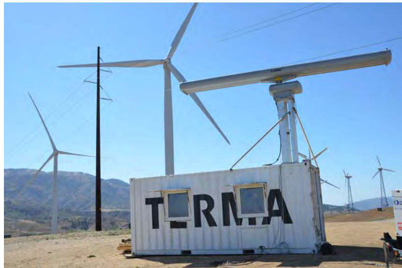
Figure 6. Terma SCANTER 5202 PSR Installed at TWRA
