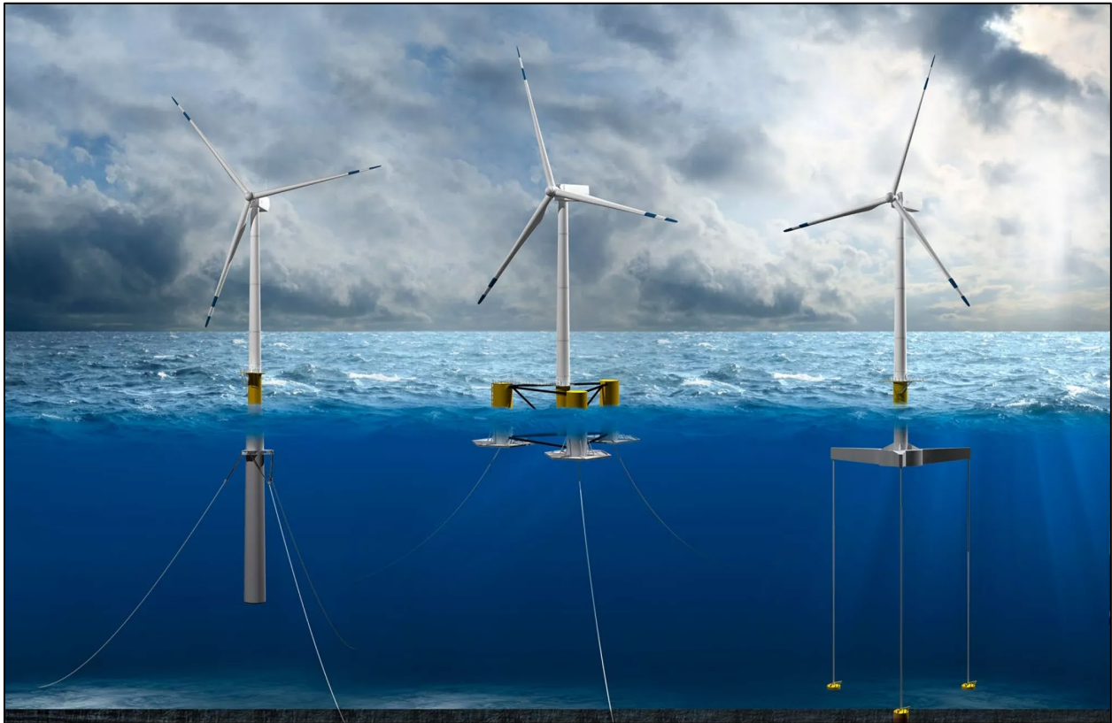
Figure 5. Illustration of floating foundation types (left to right: spar, semi-submersible, TLP) (Kreider et al. 2022 and illustration by Joshua Bauer, NREL)
