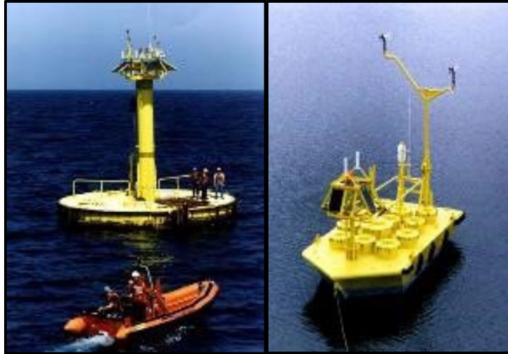
Figure 2-2: 10-Meter Discus-Shaped Hull Buoy (left); 6-Meter Boat-Shaped Hull Buoy (right)
