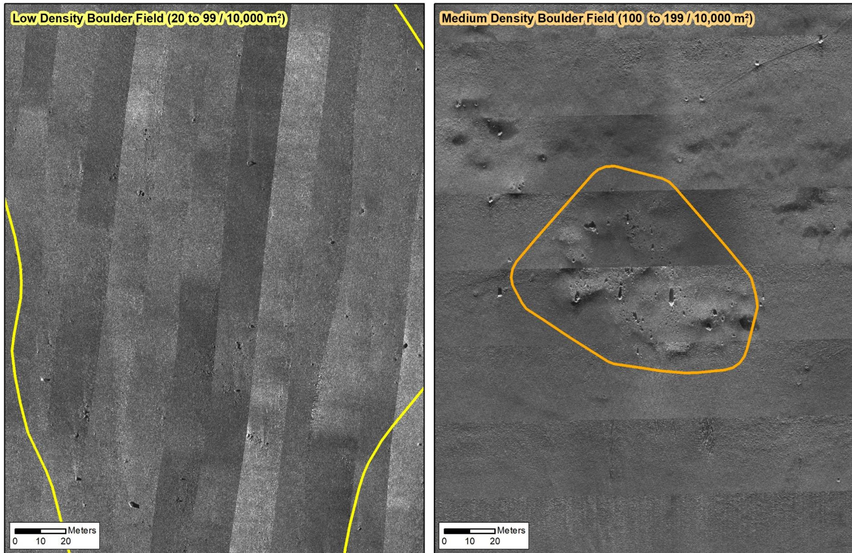
Figure 3-8. Low density (20 to 99 boulders / 10,000 m 2 ) (left) and medium density (100 to 199 boulders / 10,000 m 2 ) (right) boulder fields identified from geophysical data and included as a habitat type modifier for mud, sand, and coarse sediment habitat types where present
