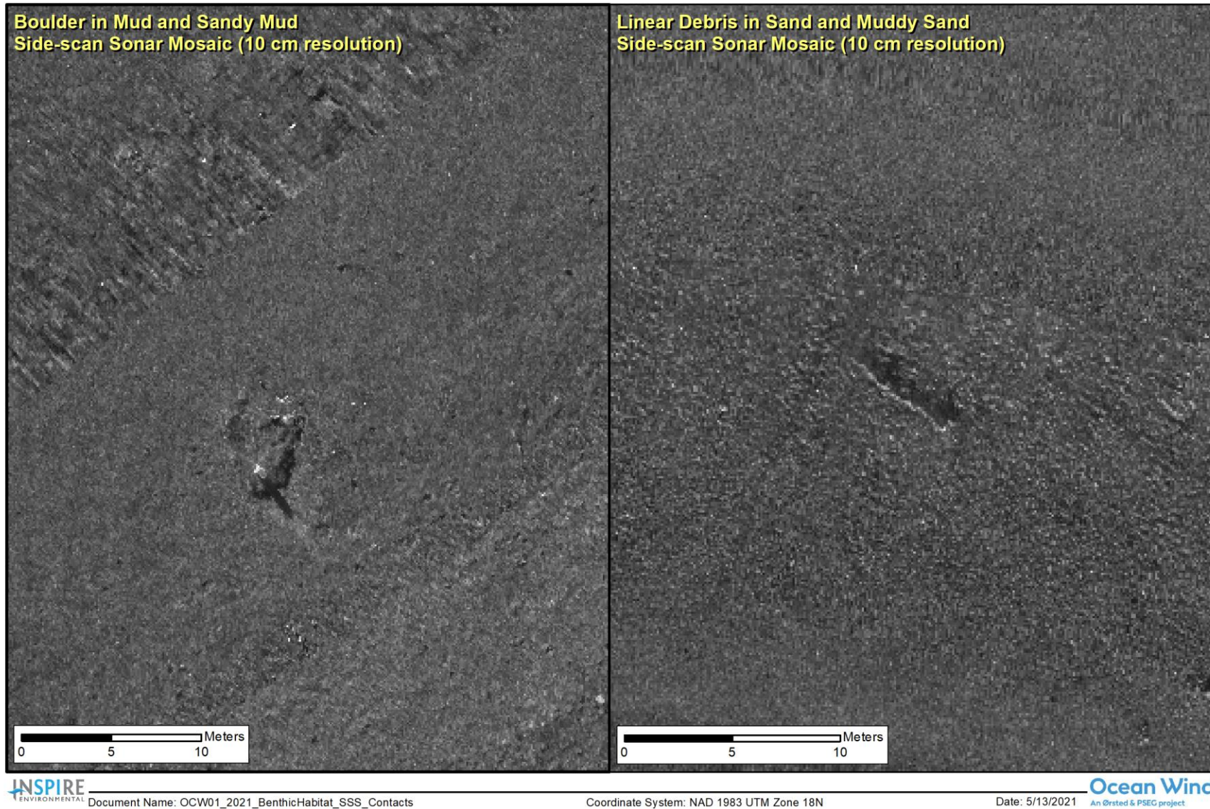
Figure 2.7. Examples of side-scan sonar data showing individual objects on the seafloor, identified as boulders (left) and debris (right)
