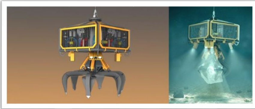
Figure 3.3.3-5 Typical Boulder Grab Configuration
