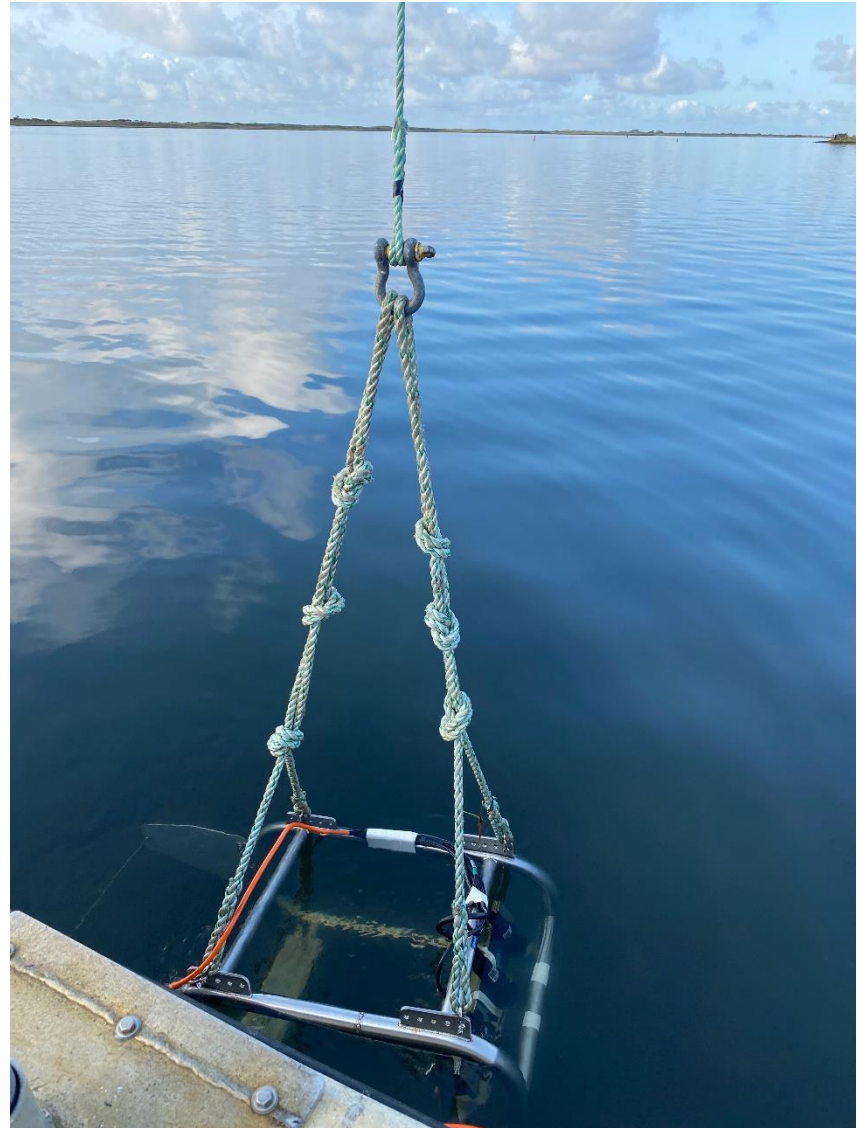
Figure 2.3-1 Photographs of the video sled used during the ICW survey to collect video footage in order to detect the presence and extent of submerged aquatic vegetation (SAV) within 100 m of the planned HDD route
