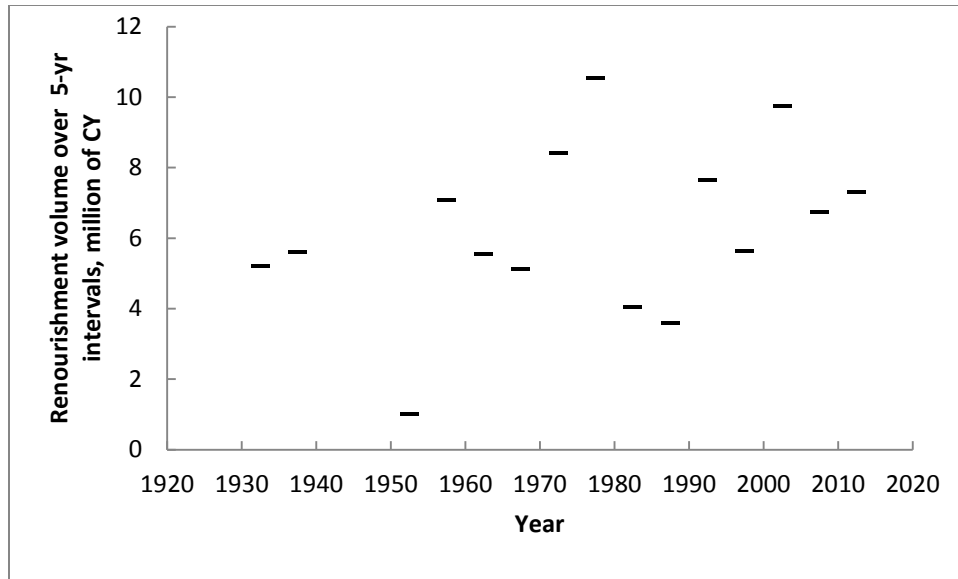
Figure 2. Total renourishment volumes over five-year intervals from a merger (Appendix 2) of ICES, Kana (1995) and BOEM records discussed in the text.
