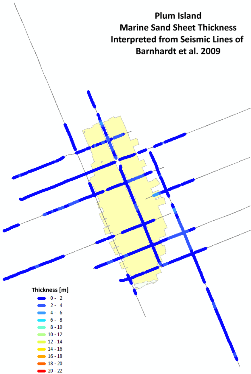
Figure 30. Estimated thickness of mobile marine sand sheet at the Plum Island site based on re-interpreted seismic data collected by Barnhardt et al. (2009).
