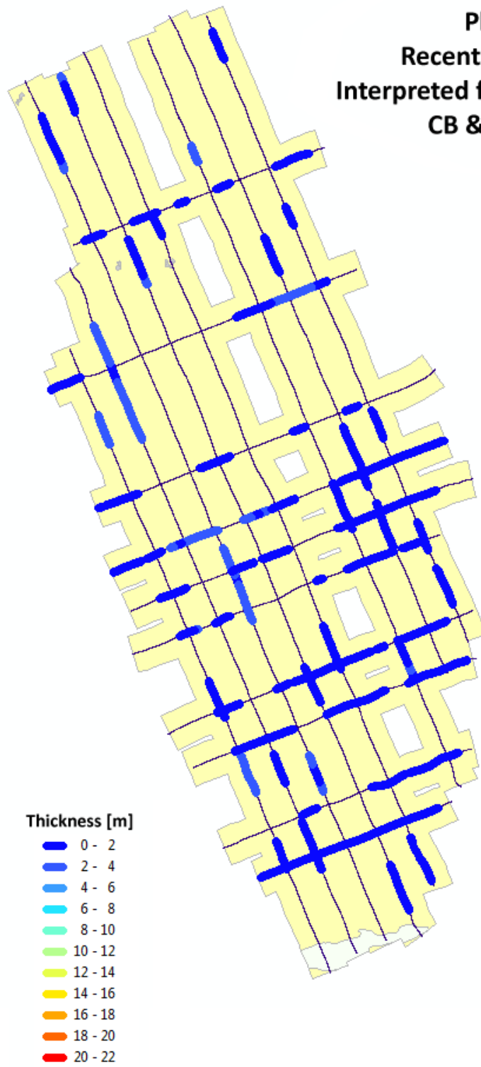
Figure 34. Estimated thickness of mobile marine sand sheet at the Plum Island site based on interpreted seismic data collected by CB&I in 2015.
