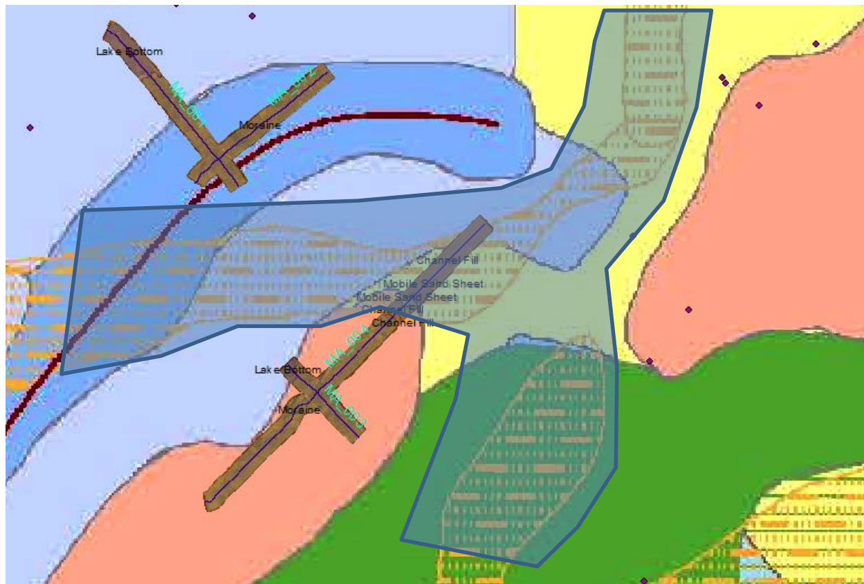
Figure 10. Area outlined in blue shows the location of channel fill deposits in the Buzzards Bay area that may warrant additional investigation. Also shown is 300 kHz side scan sonar data collected as part of this study overlain on the draft Quaternary geologic map of Massachusetts (colored polygons).
