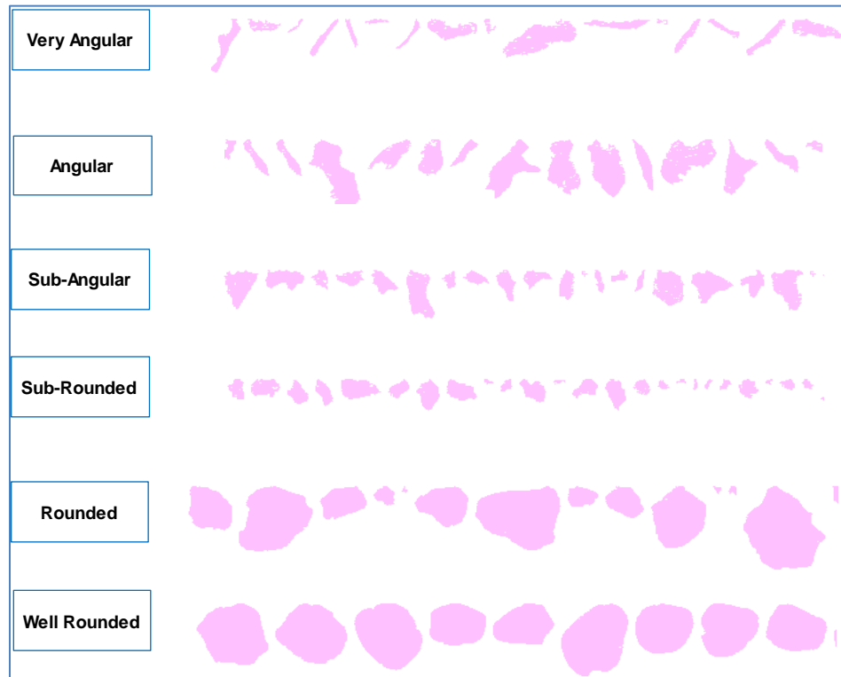
Figure 52: Shape Factor Illustration of Particles
