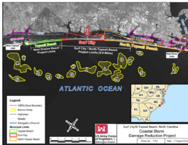
Figure 19: Map of sand management projects and potential offshore borrow areas (from Civil Works Review Board Presentation on USACE, 2017). Note, several previously identified borrow areas (I,K,M,R) were excluded based on sidescan sonar mapping results (USACE, 2010), and Borrow Area X, is not shown as it was identified later.
