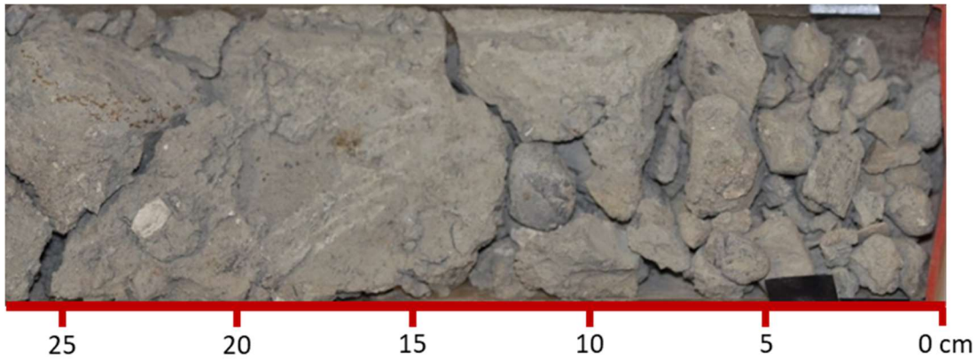
Figure 11. Photograph of vibracore UNH-2 from the surface to ~0.26m. Note pebble lag deposit at the surface of the core. The sediment below the pebbles is broken up due to desiccation.
