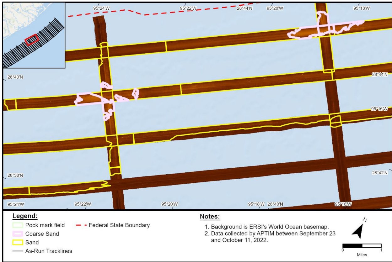
Figure 34. Highly Reflective Coarse Sand Bodies in the Sidescan Sonar Data
