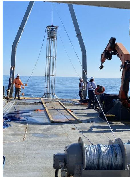
The vibracore unit was winch and A-Frame deployed and retrieved from the R/V Rachel K Goodwin. The vibracorer's light weight modular construction allowed for a safe and efficient deployment and retrieval to and from the survey vessel. The vessel "live boated" at all geologic sample locations to reduce and mitigate any potential bottom disturbance.
